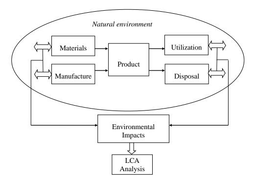
Fig. 4. Relation: product – environment in the LCA methodology.
